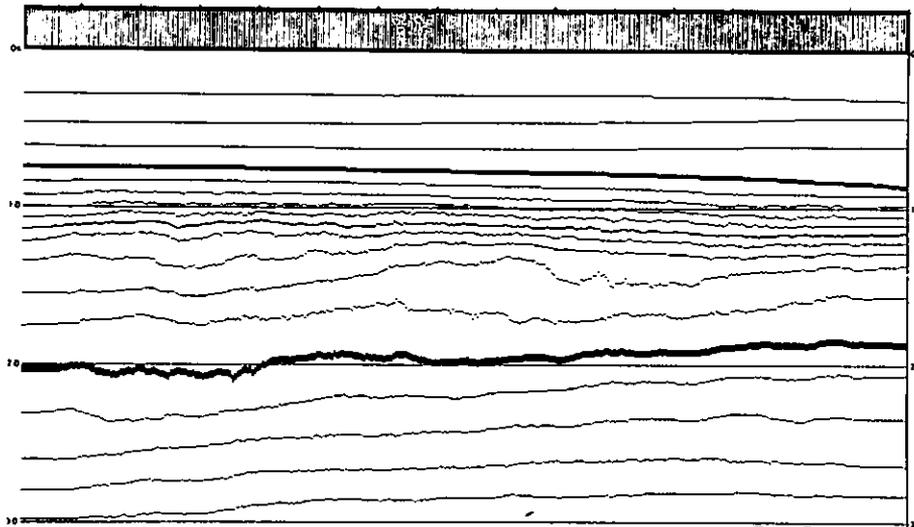
fig. 4 Isoline presentation of stacking velocities automatically calculated from field traces
