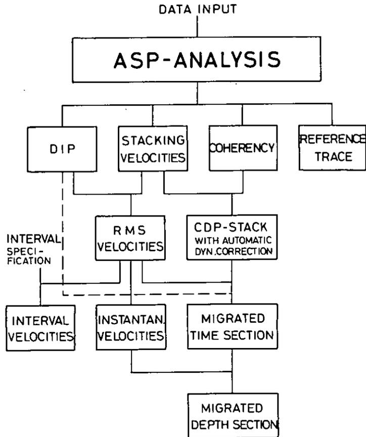
fig. 14 Block diagram of the procedure
