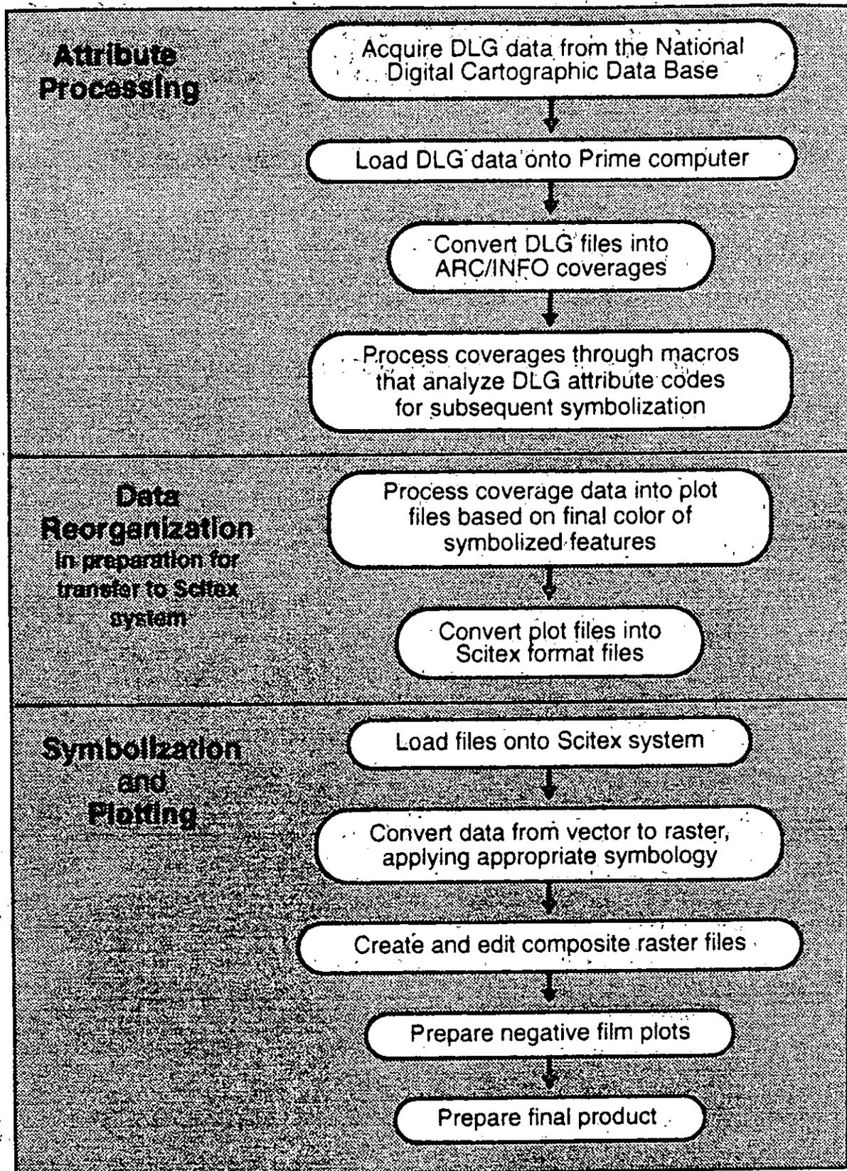
Figure 1. Outline of the process developed to generate graphic products from Digital Line Graph data.
